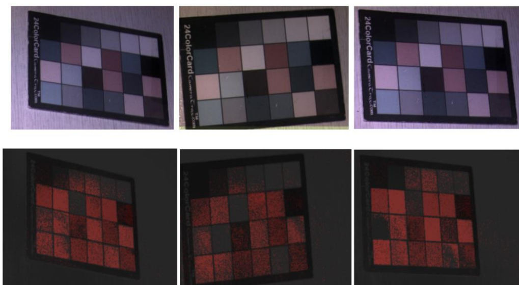
Figure 4. The 24-colormap captured using the hyperspectral camera. The three images on the top represent the 24-colormap at different angles where RGB images are false-colored for better visibility. The bottom three images represent the original hyperspectral black and white images overlaid with the segmentation results in red.
