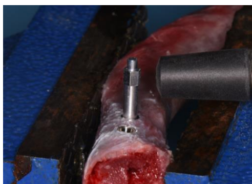
Figure 4. Registration of the implant stability quotient.
