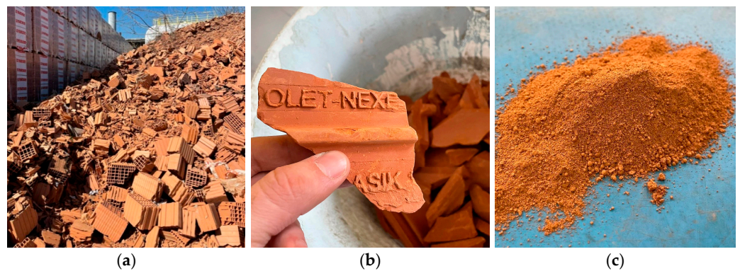
Figure 2. (a) Ceramic manufacturing waste. (b) Crushed clay blocks. (c) Ceramic waste powder, after grinding.
