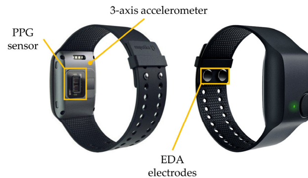
Figure 1. Insight of the relevant sensors positions in Empatica 4.
