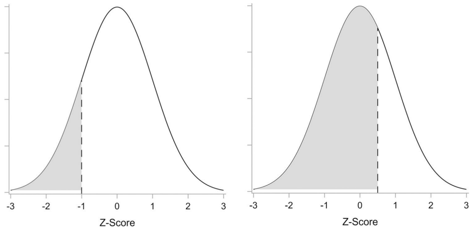
Fig. 1. Plots showing how probit scale uses area under a standard normal distribution to determine predicted probabilities. The left panel shows the predicted probability of y = 1 as the grey shaded area to the left of a Z -score of -1 . The right panel shows the predicted probability that y = 1 as the grey shaded area to the left of a Z -score of +0.50 . The predicted probabilities for y = 0 based on thresholds are represented by the white space under the curve
