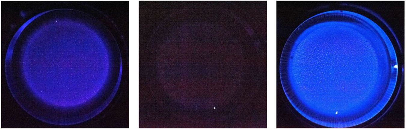
Figure 4. Uniform nspsDBD in (left) air, (middle) pure oxygen, and (right) pure nitrogen. Images were captured with a Nikon D700 at the following settings: 25600 ISO speed, f/4.5, 1/40 s exposure time, +5 step exposure bias, and 105 mm focal length. Plasma was generated by applying a high voltage pulse of 29 kV over a 1 mm gap distance. Differences in light intensity may be due to the different emission wavelengths from the gases.
