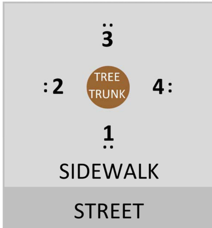
Figure 1. Diagram of the protocol for sampling methane and oxygen concentrations in sidewalk tree pits. The black dots represent the two adjacent holes, one for the methane sample and one of oxygen sample, that were created at each of the four locations around the tree trunk.
