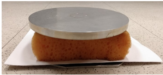
Figure 3. Colony imprinting tool. The imprinting tool consists of a 3/8" steel plate, flat sponge, folded A4 paper, filter paper with colonies, MALDI target plate, and protective steel plate, from top to bottom.
