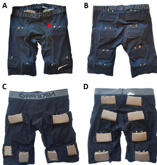
Fig. 1 A, B Pants from the outside ( A frontside, B backside), seen are the connectors for external junctions. C, D Inside of the pants ( C frontside, D backside). Seen are the side of the electrodes that are applied to the skin, the larger electrodes are sized 5 \times 9 cm (upper electrodes in C and all electrodes in D ) and the smaller (lower electrodes in C , which were used in this study) are sized 5 \times 5 cm. The red “X” in picture A demonstrated the approximate location of the ultrasound probe. The pants are thigh fitting and were adjusted so they had good contact with the skin for all participants
