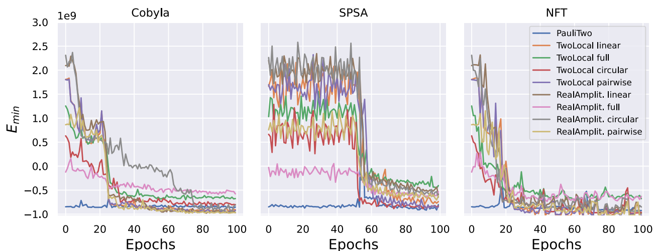
Figure 3. Noisy experiments, performed on IBM QASM simulator, by importing IBM Cairo quantum computer noise model. Convergence of the solutions towards the optimal one during training epochs, evaluated with different optimizers and ansatzes. For all these experiments, a penalty term \lambda = 10 was used.
