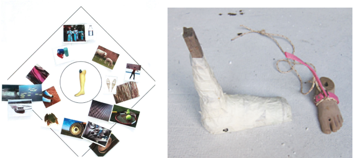
Figure 3. Co-design process of a prosthetic device for children in rural Cambodia. ( Left ) Co-design participants selected images to inspire the design of their desired product, including factors related to functionality (e.g., lightweight, waterproof) and aesthetics (e.g., brightly colored). ( Right ) An early prototype co-designed with diverse stakeholders that included a string attached to the foot that could be pulled if the prosthetic became stuck in the mud (a key concern among end users). Figure reproduced from Reference 96 (CC BY-NC-ND 4.0).
