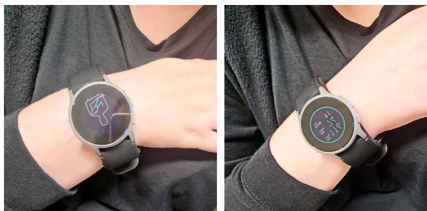
Figure 2. Measurement procedure: The device is positioned at heart level in accordance to the instructions on the display ( left ); after the measurement, blood pressure values are displayed ( right ).
