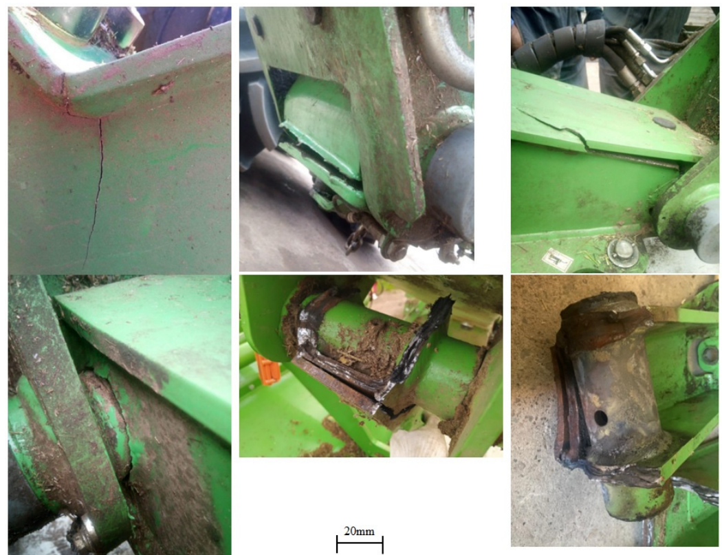
Figure 1. Operational cracks in forage harvesting machine structures made of S355 steel.
