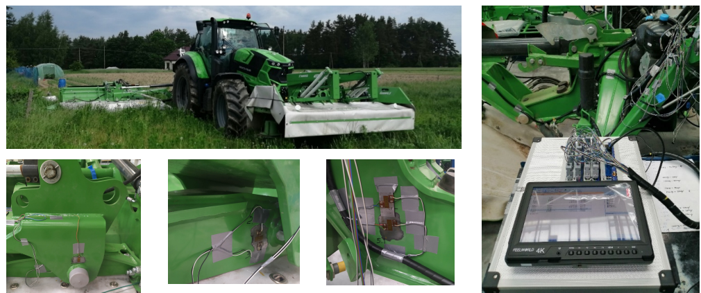
Figure 3. Test stand for determining operational loads during the grass-cutting process.
