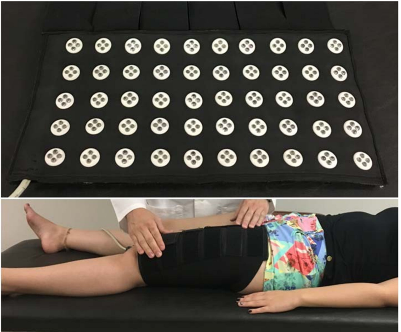
Figure 2. Light-emitting device composed of 200 low-intensity LEDs (light-emitting diodes), containing 25 arrays of 4 LEDs in the red range and 25 arrays of 4 LEDs in the near-infrared range. Only near-infrared light was used in this study. Example of irradiation on the quadriceps femoris muscles.
