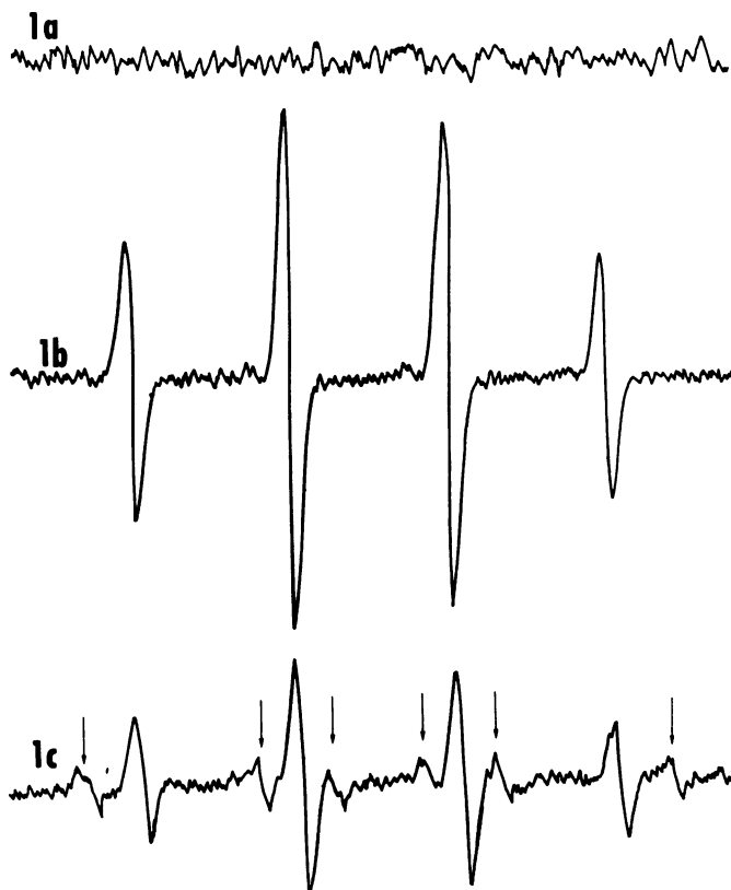
FIG. 1. First derivative ESR spectra of the spin-trapped free radicals produced when ozone is blown over a 10 mM phosphate buffer (pH 7.2). a, Typical noise generated when no radicals were produced. Ozone was blown over the phosphate buffer but no caffeic acid was present. b, 1:2:2:1 spectrum obtained with 0.5 \times 10^{-4} M caffeic acid present and 60 s of ozone exposure (0.3 \mu\text{g/g} dissolved ozone). c, Spectrum obtained under same conditions as 'b', but with 0.45 M sorbitol present. Arrows indicate a separate six-line spectrum which is a sorbitol adduct.
