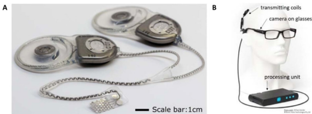
Fig. 8 The Generation 2 by Bionic Vision Australia (BVA) A: Internal components B: External components (Reprinted with permission from Petoe MA, Titchener SA, Kolic M, Kentler WG, Abbott CJ, Nayagam DAX, et al. A Second-Generation (44-Channel) Suprachoroidal Retinal Prosthesis: Interim Clinical Trial Results. Transl Vis Sci Technol. 2021;10(10):12.)
