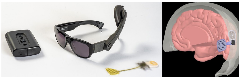
Fig. 9 The ORION Visual Cortical Prosthetics system. External components (Left). It is placed on the medial occipital lobe over V1 and V2 (Right) (Courtesy of Gislin Dagnelie, Ph.D.)
