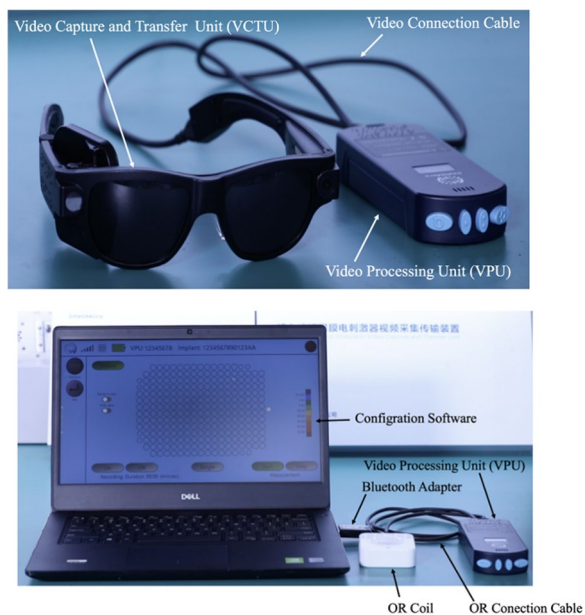
Fig. 3 External component of the IMIE 256 (Modified and reprinted with permission from Xu H, Humayun MS, et al. First Human Results With the 256 Channel Intelligent Micro Implant Eye (IMIE 256). Transl Vis Sci Technol. 2021 Aug 12;10(10):14.)
