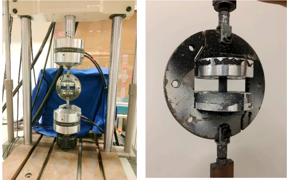
Figure 4. Experimental set-up of adhesive connections subject to Mode I loading by means of an Arcan-modified device.
