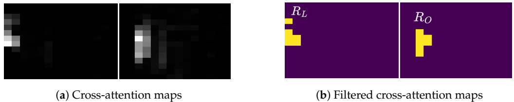
Figure 5. The estimated character locations, R_k , for the two predicted characters of the input image in Figure 4a, from the cross-attention maps. (a) Cross-attention maps. (b) Estimated character regions. Best viewed in color.
