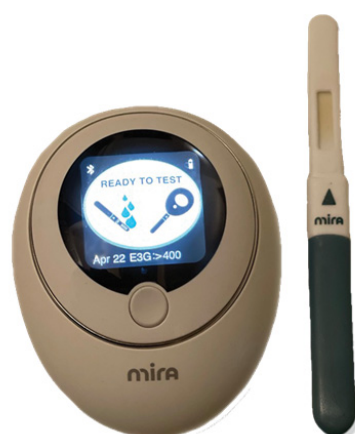
Figure 1. The Mira Analyzer measures follicle-stimulating hormone (FSH), estrone-3-glucuronide (E 1 3G), luteinizing hormone (LH), and pregnenediol glucuronide (PDG) in the urine. It is comparable in identifying hormone changes to the well-known ClearBlue Fertility Monitor. This figure is a partial reproduction of Figure 1 from ref. [3].
