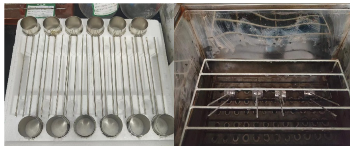
Figure 5. Rayleigh clamping boiling method for stability testing.
