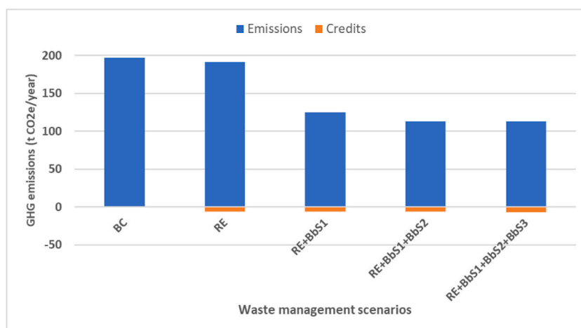
Fig. 5. GHG emissions comparison between the base case and the combined waste management scenarios.
