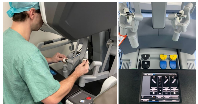
Figure 6. Da Vinci's console and surgeon's interactivity with a binocular visualization, instruments and pedals.
