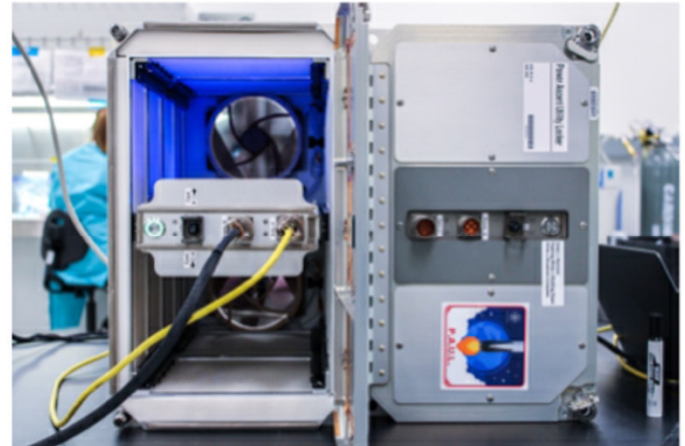
Supplementary Figure 2: CubeLab (top and bottom-left) facility that will house the vibrational bioreactor and the biological samples. The PAUL (top and bottom-right) facility designed to house and provide mechanical, electrical, and network interface from the outside
