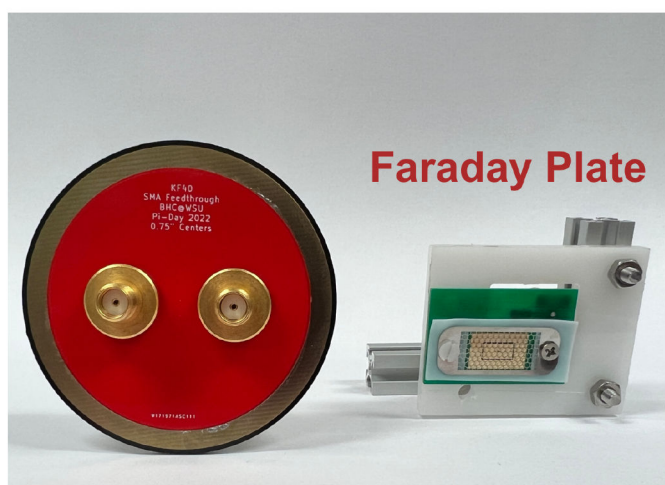
Figure 5. The top set of images, a.), highlights the two-board infrastructure that allows for the assembly of a KF40-compatible electrical feedthrough that accommodates hermetically sealed SMA, BNC, or a 10-pin IDC connector. By sealing the smaller board with heated solder paste to a larger ring, the completed board set directly fits with a KF40 centering ring (lower right of a.)). b.) shows a completed SMA board and a separate solution for recording SLIM separations using a Faraday plate customized to the SLIM environment. All files for these boards are provided in the Supporting Information and via github.
