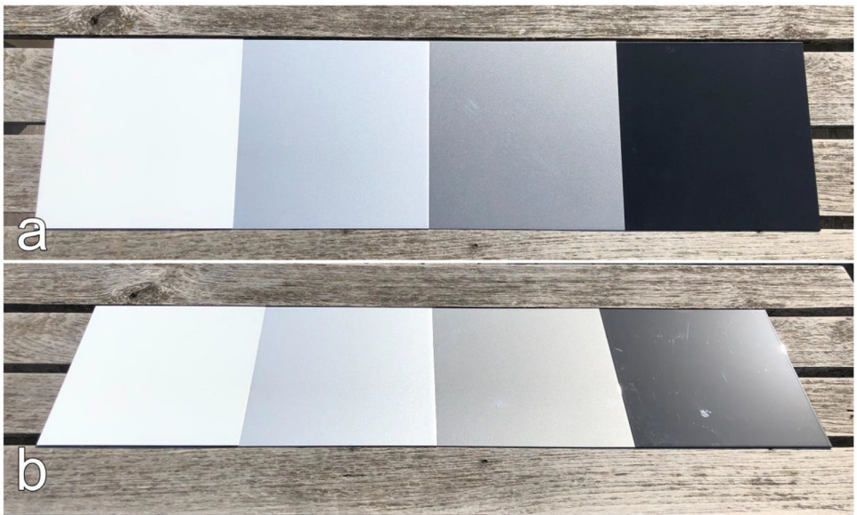
Fig. 6. Glossy vehicle varnish samples in different greyscale – white, silver (metallic), grey (metallic), black – arranged in line to give an impression on their reflective behavior in the optical spectrum. (a) top view. (b) tilted view.
