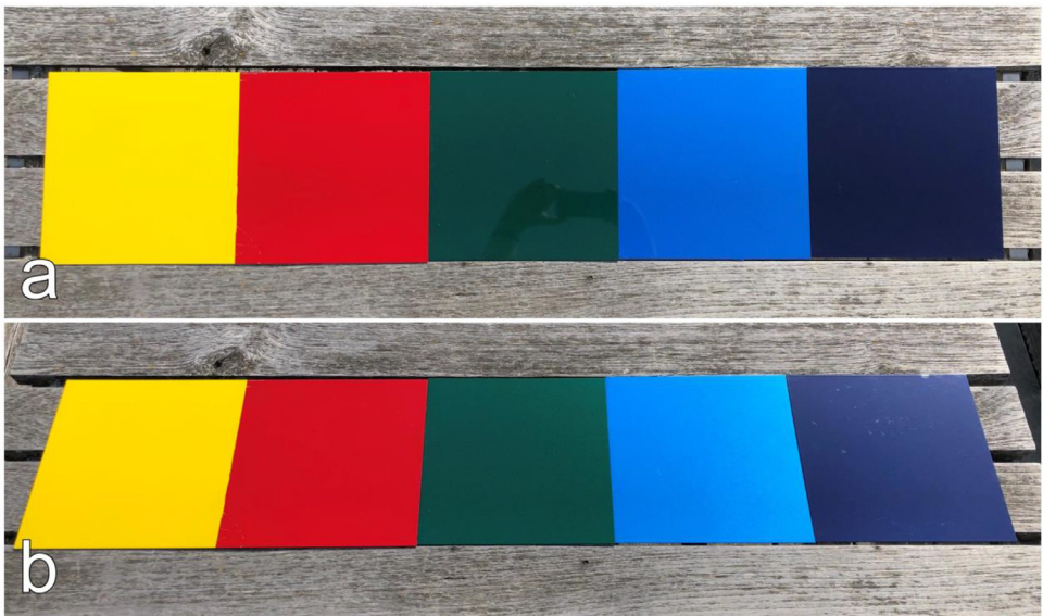
Fig. 4. Colored vehicle varnish samples arranged in line to give an impression on their reflective behavior in the optical spectrum. The yellow and red samples are of solid color type whereas green, blue, and dark blue are of metallic type. (a) top view. (b) tilted view.
