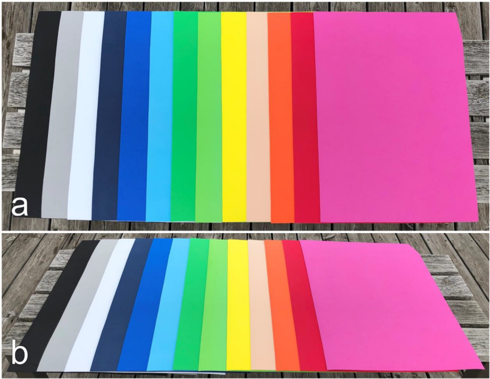
Fig. 7. Three greyscale and ten color moss rubber samples arranged overlappingly in line to give an impression on their reflective behavior in the optical spectrum – black, grey, white, dark blue, blue, light blue, dark green, green, yellow, beige, orange, red, pink (from left to right). (a) top view. (b) tilted view.
