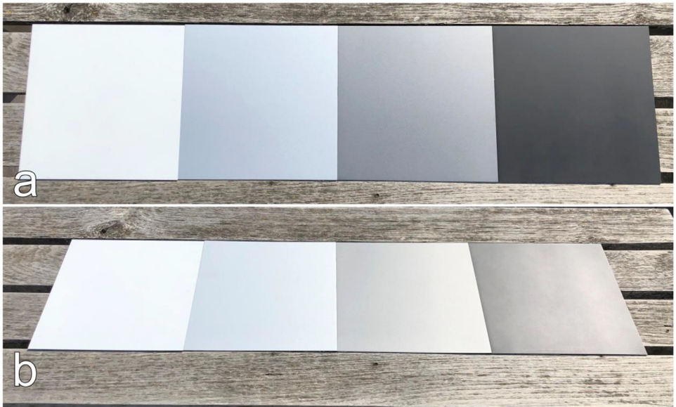
Fig. 5. Mate vehicle varnish samples in different greyscale – white, silver (metallic), grey (metallic), black – arranged in line to give an impression on their reflective behavior in the optical spectrum. (a) top view. (b) tilted view.
