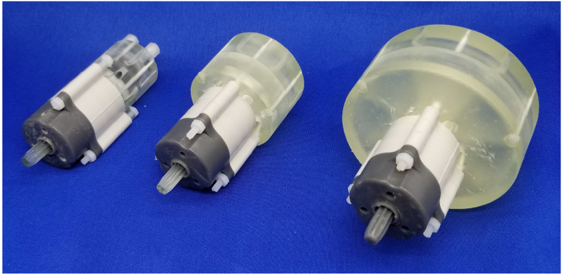
Fig. 1. Three different scaled motor designs. (Left) Motor with 19 mm OD rotor (authors' nominal preference). (Center) Motor with 44 mm OD rotor (motor size from [18]). (Right) Motor with 61 mm OD rotor.
