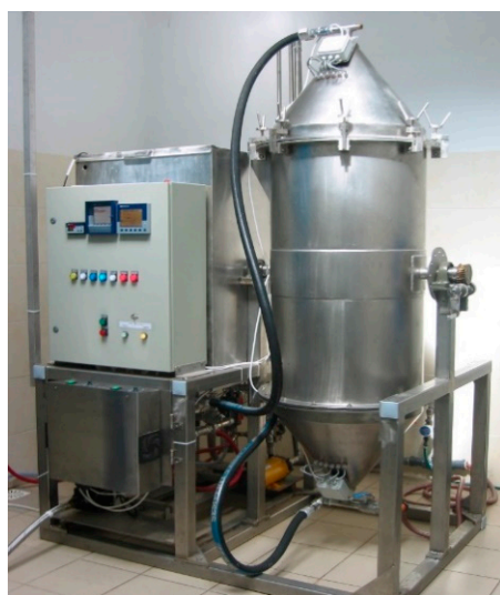
Figure 1. Prototype device for osmotic degumming of fibers in a periodic raw material loading system, built using LIST in Poland.
