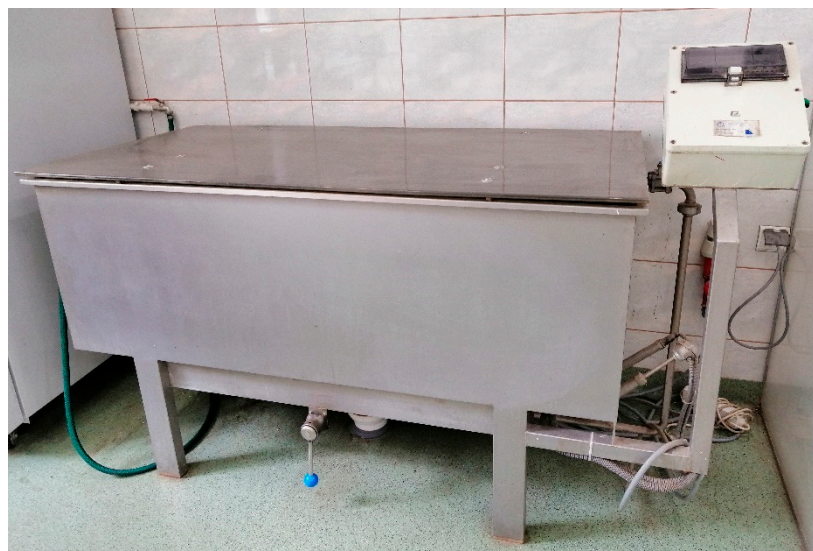
Figure 4. Prototype device for water retting of straw, built by LIST in Poland.
