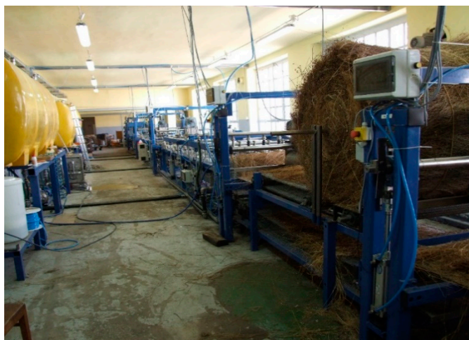
Figure 2. Prototype device for osmotic degumming of fibers in a continuous raw material loading system, built using LIST in Poland.
