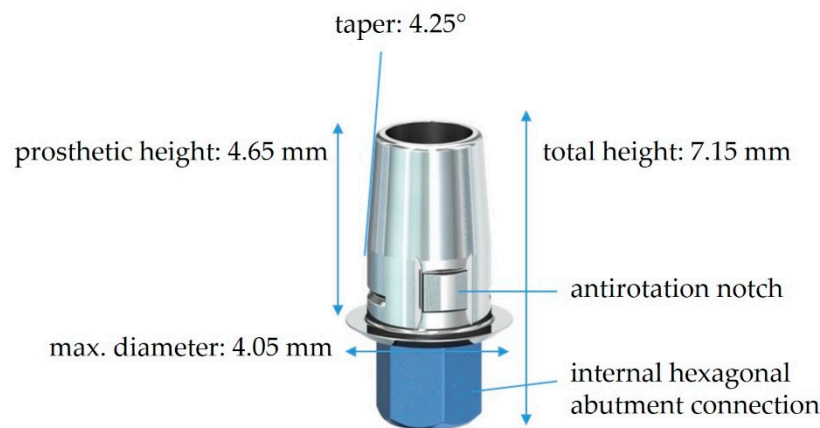
Figure 3. The specifications of the titanium bonding base straight CAD/CAM used in the current study (image source: https://shop.sic-invent.com/en , accessed on 16 November 2023).
