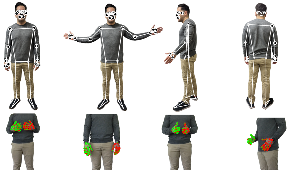
Figure 3. HARE's adaptability to different use cases is demonstrated by leveraging diverse landmark estimation models. The top row shows examples of 2D pose estimations, while the second row illustrates hand landmarks with specific annotations (e.g., right hand with red circles and green connection lines, left hand with green landmarks and red connection lines). By utilizing different models, HARE can accommodate a wide range of applications.
