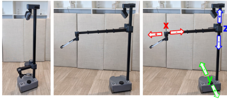
Fig. 3. Modes offer insight (left to right): navigation mode; manipulation mode; axes of Cartesian motion for the manipulation mode.
