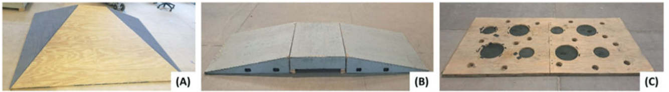
Fig 2. Driving tasks simulating non-ADA-compliant surfaces: (A) curb cut, (B) 10° ramp, and (C) series of potholes.
