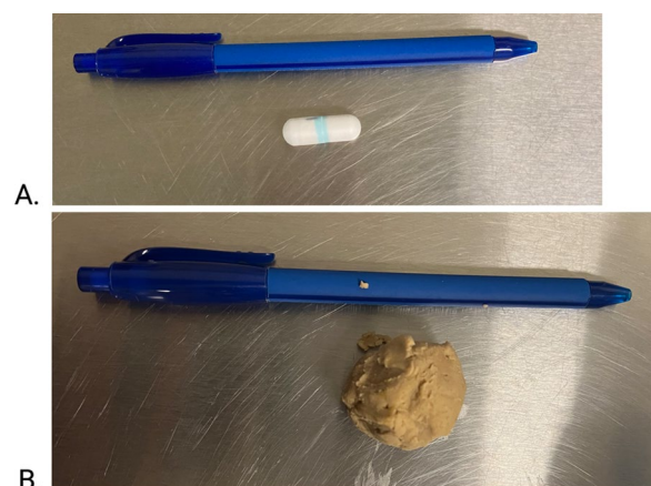
Fig. 10 A. Engineered Small Intestinal MicroBiome Aspiration (SIMBA™) capsule (Nimble Sciences) with a ball pen for size comparison. B. SIMBA™ capsule placed in a meatball of can food (Royal Canin Veterinary®, hypoallergenic hydrolyzed protein loaf, Mars inc. Puslinch, Ontario)
