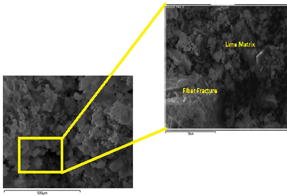
Figure 11. SEM image of hemp limecrete at hemp 6%.
