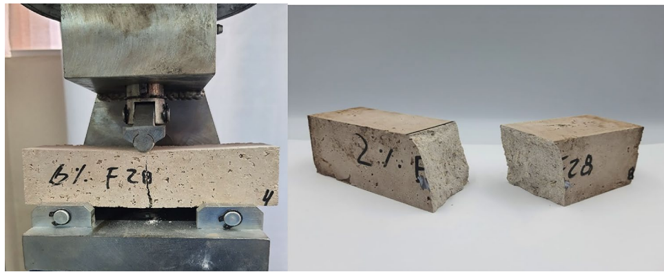
Figure 6. Flexural testing of hemp limecrete.
