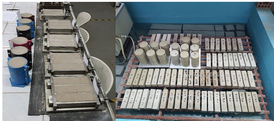
Figure 3. Casting and curing of specimens.
