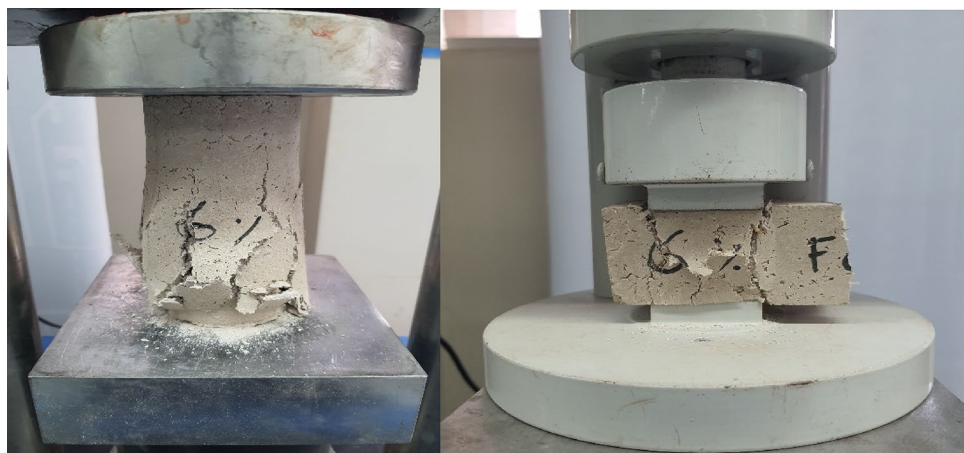
Figure 7. Compression testing of hemp limecrete.
