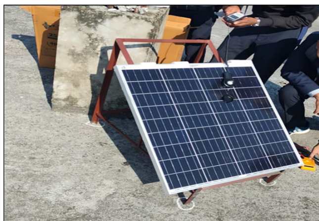
Figure 1. Solar panel test rig installed on the roof of a two-story building.
