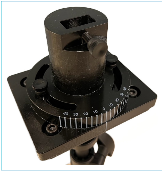
Figure 8. Rotating mount for testing angular dependence of light emitter.
