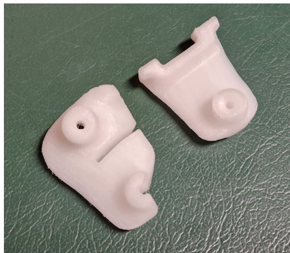
Figure 6. Example of guide design for the use of instrumentation employed with different directions (left) and for the use of instruments being used along the same direction (right).
