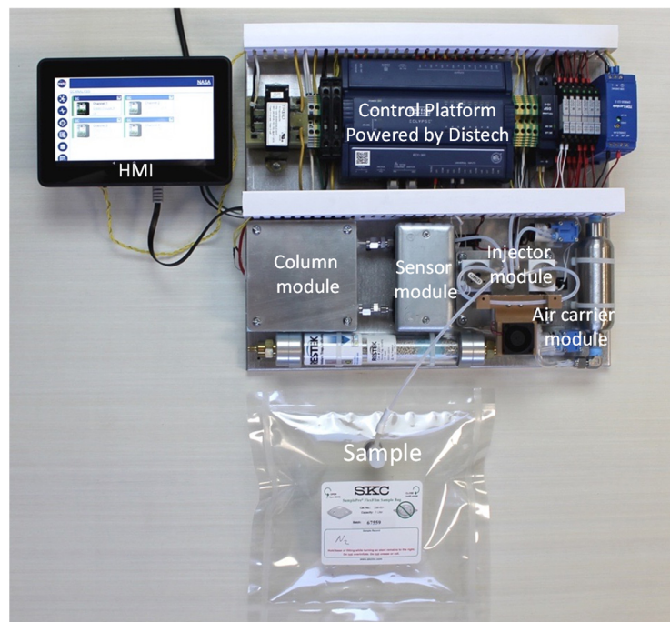
Figure 11. Structural optimization of GC components.
