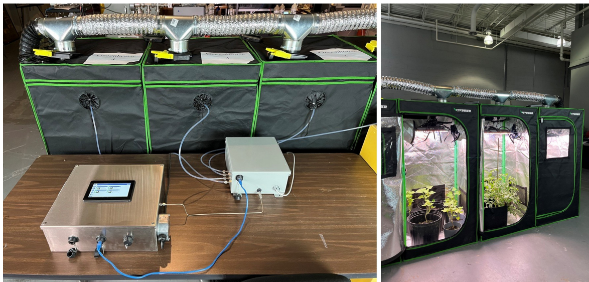
Figure 13. Monitoring of four compact greenhouses with a single chromatograph equipped with a multichannel gas sampling system.
