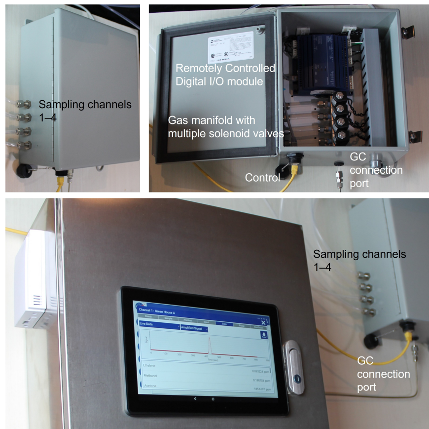
Figure 12. Multichannel gas sampling system for monitoring multiple greenhouses.
