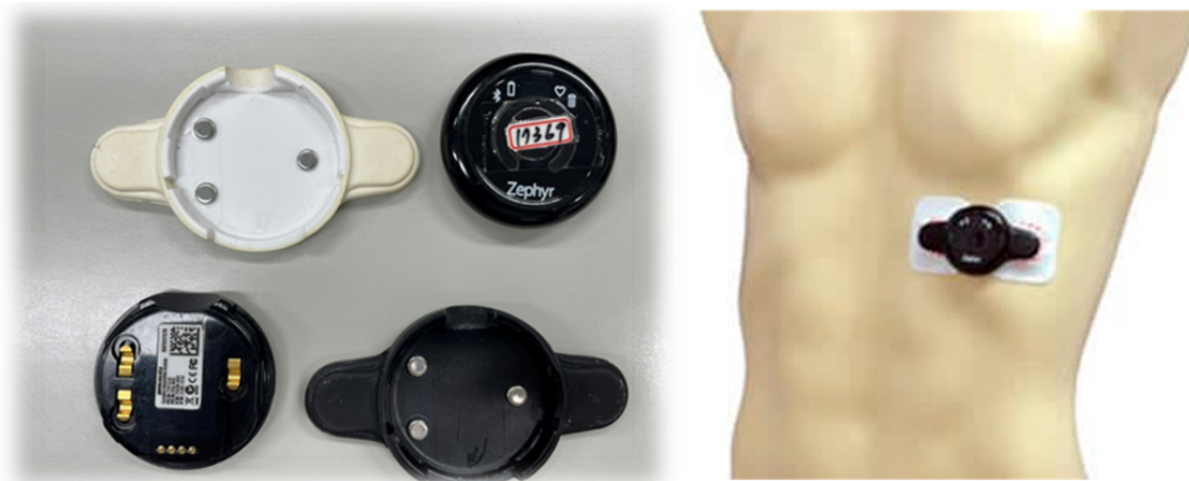
Figure 2. Schematic illustration of the BioHarness 3.0 BioPatch device and its placement.
