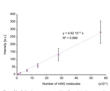
503 Figure S2 - Calibration curve between mNeonGreen intensity measured by spectrofluorometry (in arbitrary units, a.u.) 504 and the number of mNeonGreen molecules. The equation of the linear trendline, as well as the correlation coefficient 505 (R<sup>2</sup>), are indicated on the plot.
