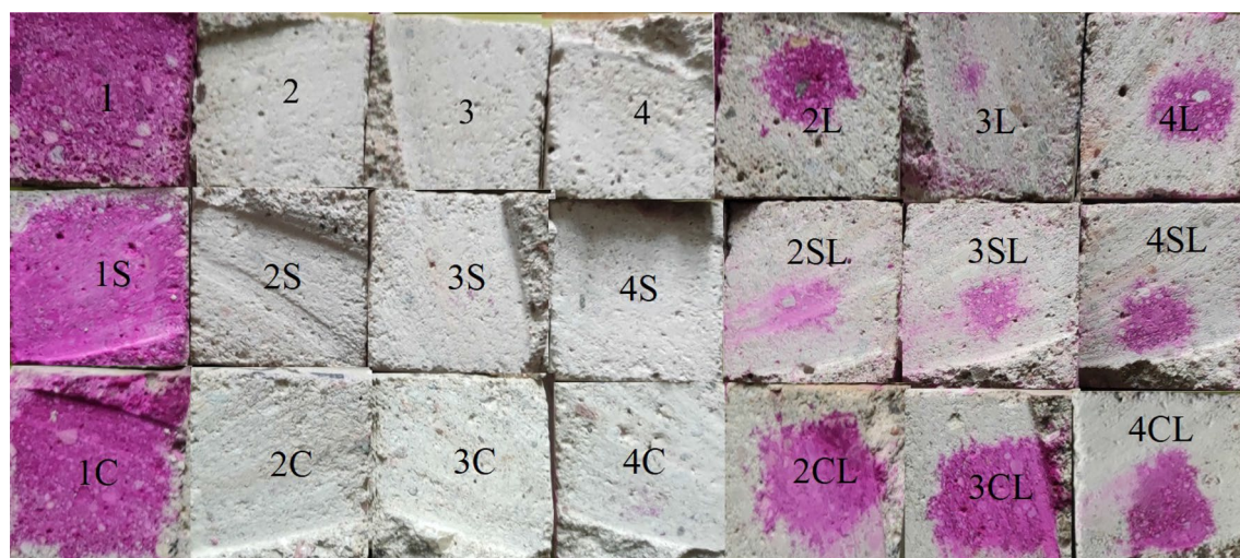
Figure 7. Results of the carbonation test after the application of phenolphthalein (violet colour indicates the presence of Ca(OH) 2 ).
