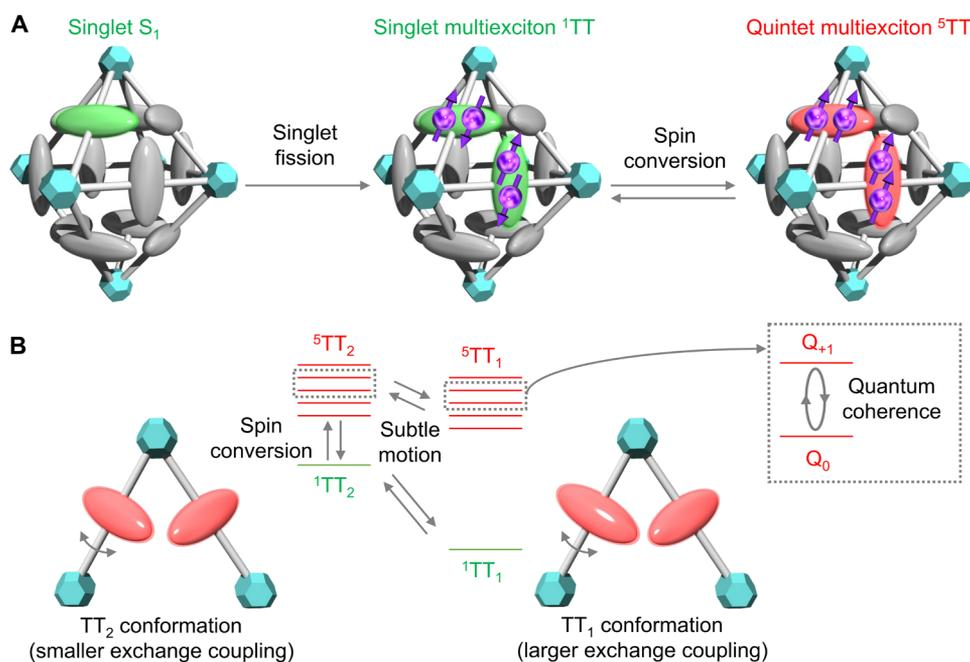
**Fig. 1. Quintet multiexciton generation and its quantum coherence in an MOF.** (A) SF followed by spin evolution via modulation of exchange interactions results in the formation of quintet multiexciton  $^5\text{TT}$  in an MOF. (B) Suppressed chromophore motion in an MOF enables not only the spin conversion from  $^1\text{TT}$  to  $^5\text{TT}$  but also the quantum coherence of  $^5\text{TT}$  over hundred nanoseconds even at room temperature.
