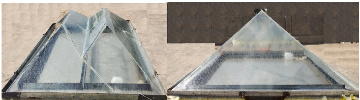
Figure (1D). Glass covers for W-shape and pyramid covers, experimental photo
