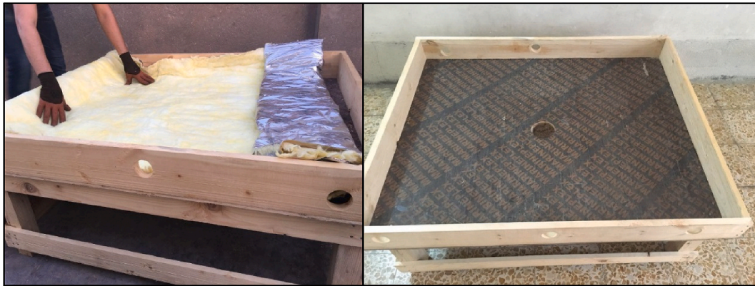
Figure 1b. glass wool insulator and wooden frame.
