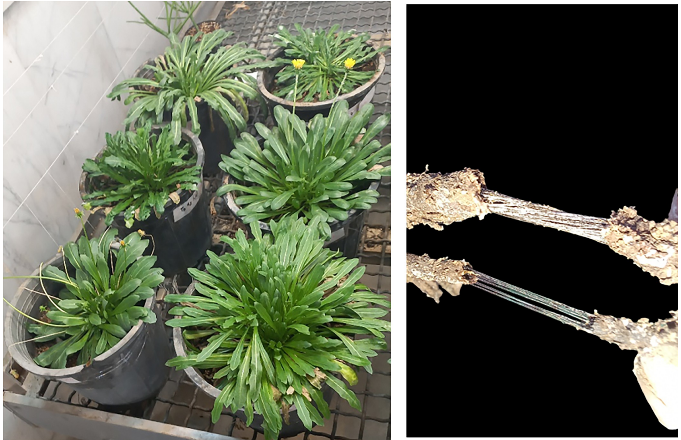
Fig 1. (a); T. kok-saghyz plants and (b); Natural rubber (TNR) strands stretched between broken root sections.
