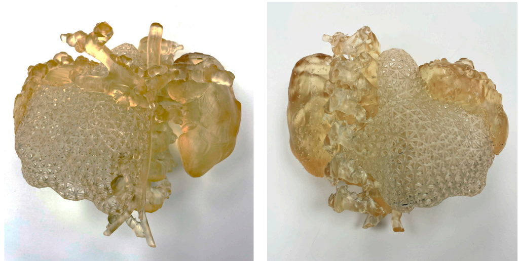
Figure 4. SLA 3D-printed model showing the anatomical parts in translucent magenta (tumor, vessels, spine and kidneys).
