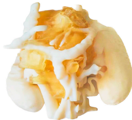
Figure 10. 3D-printed model of a sarcoma manufactured by MJ using Vero and enclosed support material. Blood vessels, heart and bronchioles are in Vero White, while the sarcoma tumor is translucent Tango Grey material.
