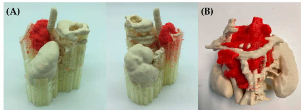
Figure 6. (A) 3D-printed realistic model showing the neuroblastoma in red in TPU and the rest of the anatomical structures (spine, vessels and kidneys) in white PLA. The other material is PVA, which is used for the support parts. (B) After the removal of the PVA, the realistic 3D-printed model is visualized [14].
