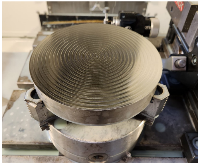
Figure 1. Workpiece material and its spiral marks.
