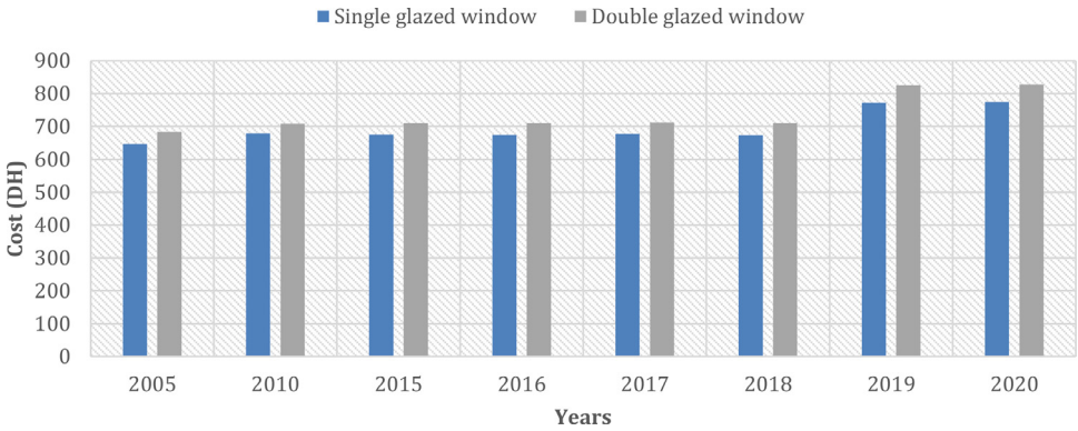
Fig 7. The evolution of the cost of windows (DH/m 2 ) in the case of single- and double-glazed windows.
