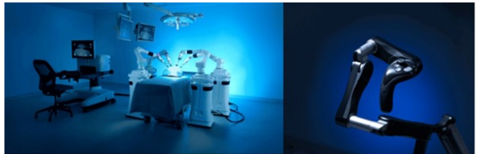
Fig. 11 Versius Surgical Robotic System, provided by and permission from CMT (left picture- surgeon console and modular bed side units, right picture- hand controller) [105]
