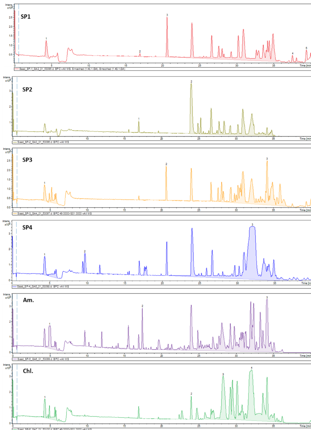
Figure 2. Base Peak Chromatogram (BPC) of the studied algal species in the positive ionization mode. Refer to Supplementary Table S3 for sample codes.
