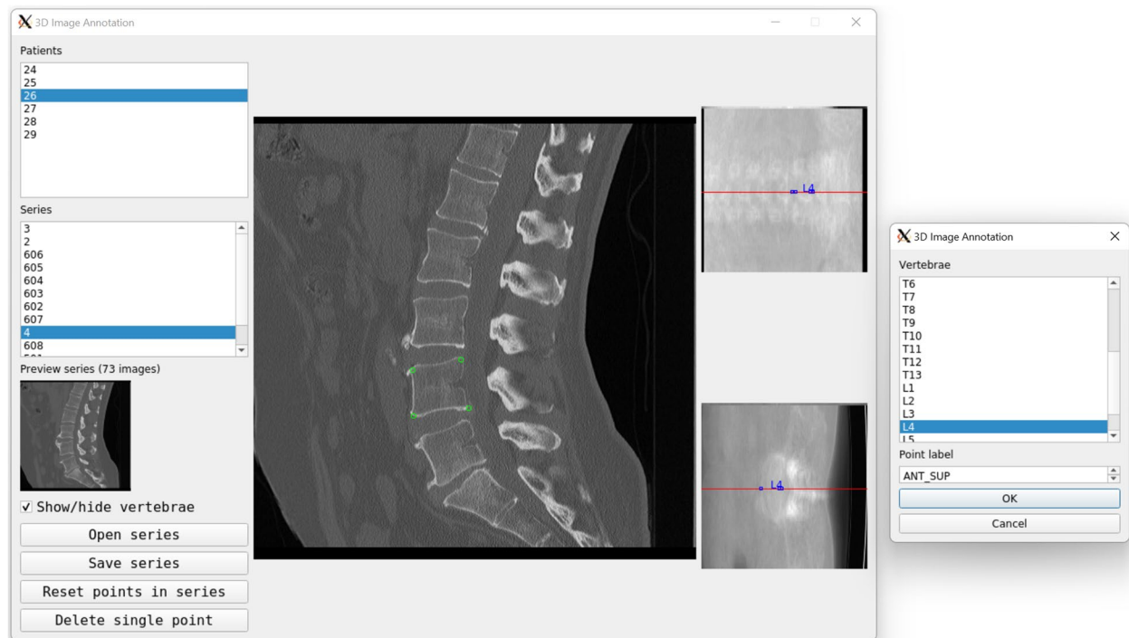
Fig. 6 Custom image annotation software developed by the authors, aimed at localising landmarks (green circles) in 3D images of the spine. This Python application runs on a local computer and does not require sharing any information over the Internet. The user interface is designed to minimise any human interaction not directly aimed at localising the landmarks on the images, considerably speeding up the annotation workflow
