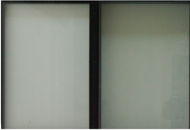
Figure 3. Photograph of the two implemented glass types: high transmittance glass/2-layered low-iron glass (left) and low transmittance glass/3-layered low energy glass (right).
